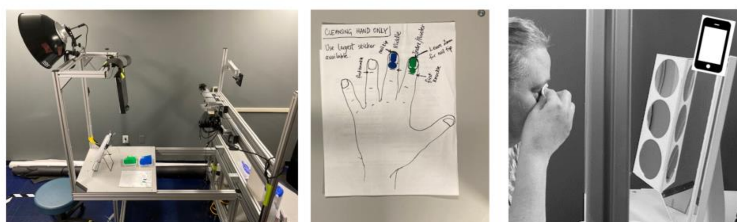
Fig -1. Video capture system with finger markers, basic lighting, with HD video recording system.
