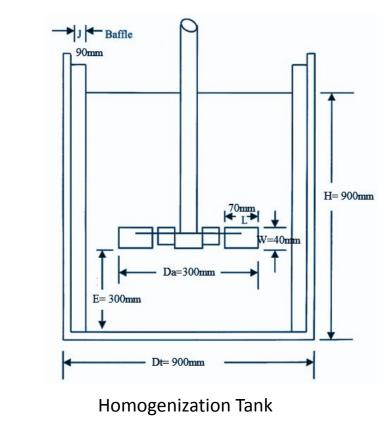
The homogenization tank was designed for 400 kg and need a 2.5 HP electric motor.
