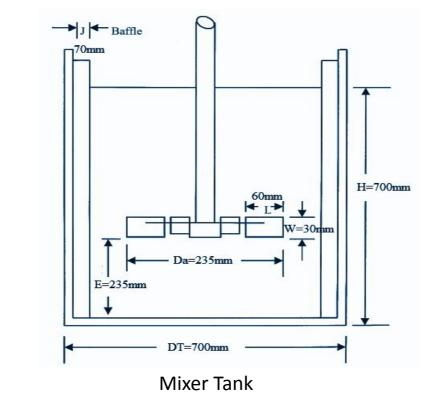
The mixing tanks were designed for a volume of 200 kg each one. Aqueous phase mixer need a 1 HP electric motor and the Oli phase mixer require a 8 HP electric motor.
